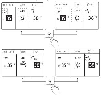
2) The unit has no DHW function or DHW mode is set unavailable.
