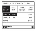
Use " <sup>(t)</sup> " to turn on/off "CURRENT STATE", and use" ▼", "▲" to adjust the operate date and start time of disinfect function.
