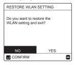
Use "◀", "▶" to move to "YES", press " ← " to restore WLAN setting. Complete the above operation and wireless configuration is reset.
