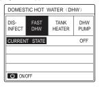
Use " O " to turn on/off "CURRENT STATE" of FAST DHW function.
