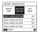
Use " O " to turn on/off the temperature curve. If "ZONE1 C-MODE LOW TEMP." is turned on, cool mode in zone 1 is activated, the following page will appear:
